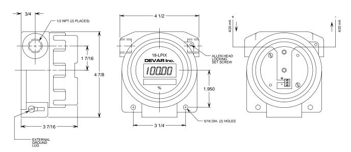
FIG. 1 GENERAL DIMENSIONS AND FIELD WIRING
